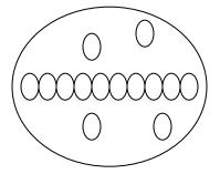
Since each object takes up 1/10<sup>th</sup> of the 2000 micrometers field of view diameter, the size of each object is 200 micrometers. You can use this method to estimate size of objects you view under your microscope once you know your microscope's field of view diameter. If two organisms fit across the field of view that has a diameter of 1000 micrometers, how large is each organism?
