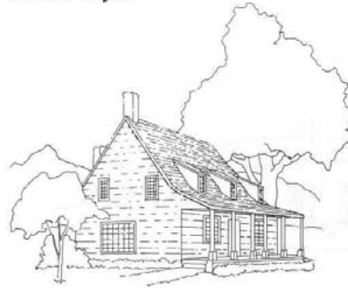
Dormers and Flared Roof
