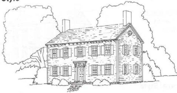
Gabled Roof, Cornice, and Fanlight
