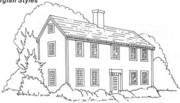
Side-gabled Roof, Cornice, and Central Chimney
