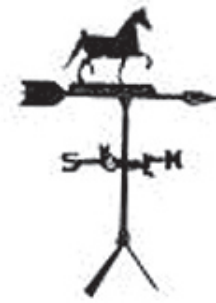
A weather vane shows the direction from which the wind is coming
