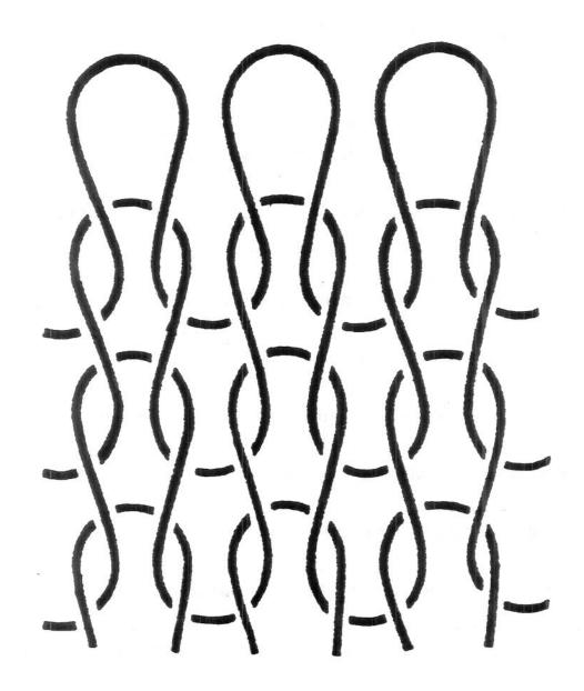
IS MADE BY A SERIES OF LOOPS FROM THE SAME, CONTINUOUS YARN, INTERLOCKED TOGETHER.
