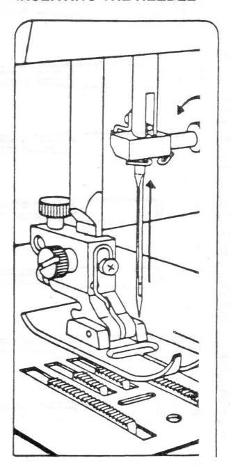
Always insert the needle with the groove facing the thread. Generally this is toward the front of the machine.
