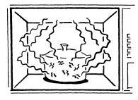
The vibration causes friction, which creates heat that cooks the food.
