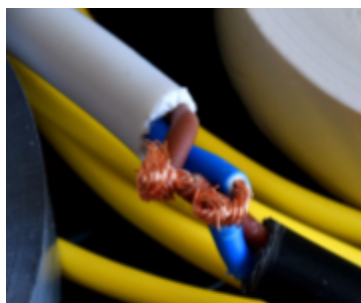
Copper wire conducts electricity while the plastic coating does not. Image by papazachariasa; pixabay.com; CC0
