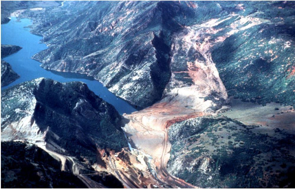
Image Aerial photo of the Thistle area in spring 1983 showing the dam formed by the landslide, "Lake Thistle" over the submerged town, and the construction to re-route US-6, US-89, and the D&RGW around the landslide area by USGS; https://en.wikipedia.org/wiki/Thistle,_Utah#/media/File:Thistlelandslideusgs.jpg ; public domain
