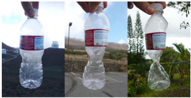
This bottle was closed at an altitude of 3,000 meters where air pressure is lower. When it was brought down to sea level, the higher air pressure caused the bottle to collapse.
