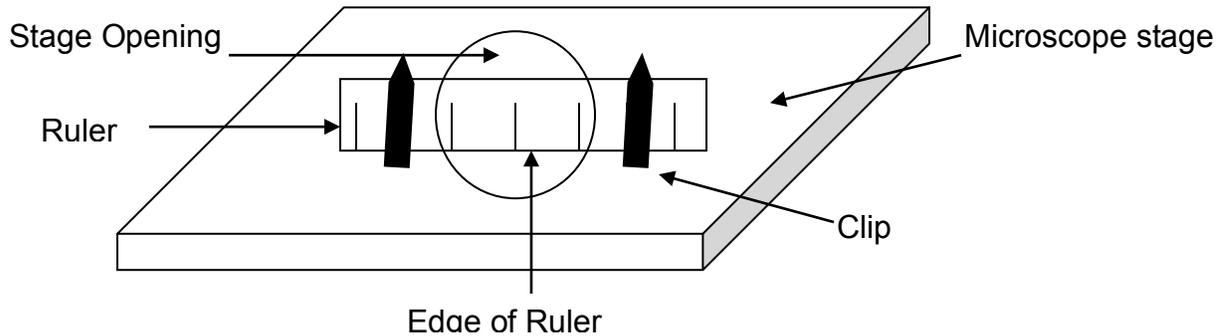
2. Position the ruler so one of the millimeter markings is just visible to the left in your field of view as shown below. Notice that the distance between the marking on the left and the next mark is one millimeter.
