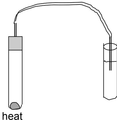
3. Heat the tube containing the  $\text{CuCO}_3$  while holding the end of the glass tube in the limewater solution with test tube clamps. Continue heating until bubbling has nearly stopped. Remove the limewater tube before removing the heat from the  $\text{CuCO}_3$ . A cloudy appearance in the  $\text{Ca}(\text{OH})_2$  indicates the presence of  $\text{CO}_2$ . Record any other observations of the products.
